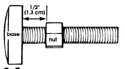
Use legs and nuts from parts package. Screw nut down to within 1/2 inch (1.3 centimeters) of base.
